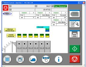
The signals of the continues batch washer and the wash extractors are connected over the Profibus modules. These signals can be interpreted as Relais or Relais enhanced. Therefore also older wash extractors can be connected too.
